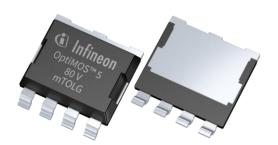
OptiMOS<sup>™</sup> 5, 80 V, 1.2 mΩ world-class low R<sub>DSon</sub>
