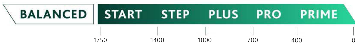
Categorization for carbon steel, in kg CO 2 e per ton of steel.
