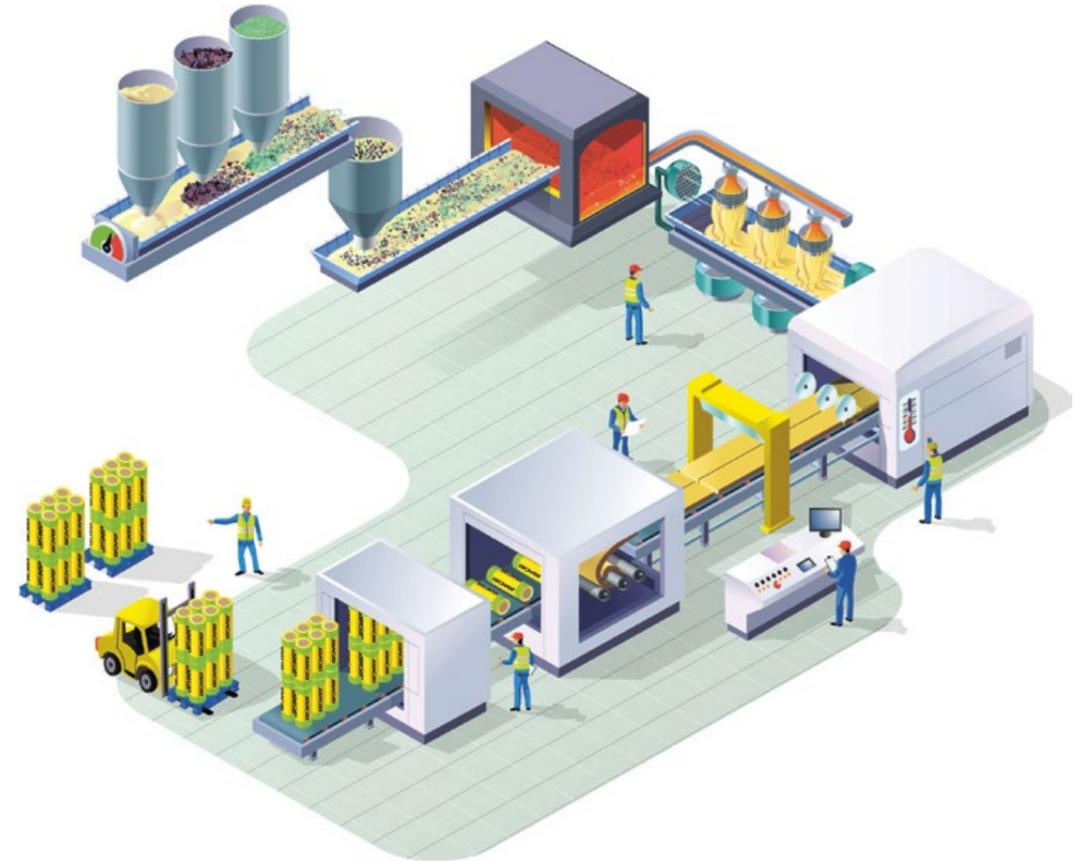
the glass wool during transport is important. That is because contact with water increases the heat conductivity of the insulation material and thus reduces its insulation capacity. Most ISOVER products can be compressed to a tenth of their volume, packed, and transported in a space-saving way. Trucks transport the pallets to HORNBAACH’s various outlets, where customers can take the rolls and packages from the shelves or opt for a HORNBAACH delivery service.
