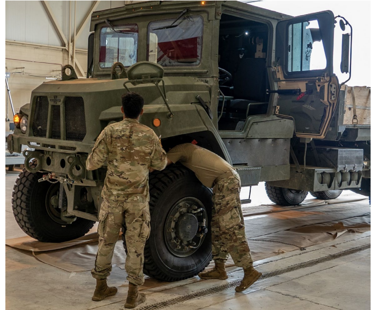
FMTV A2 LVAD Preparation for Parachute Testing
