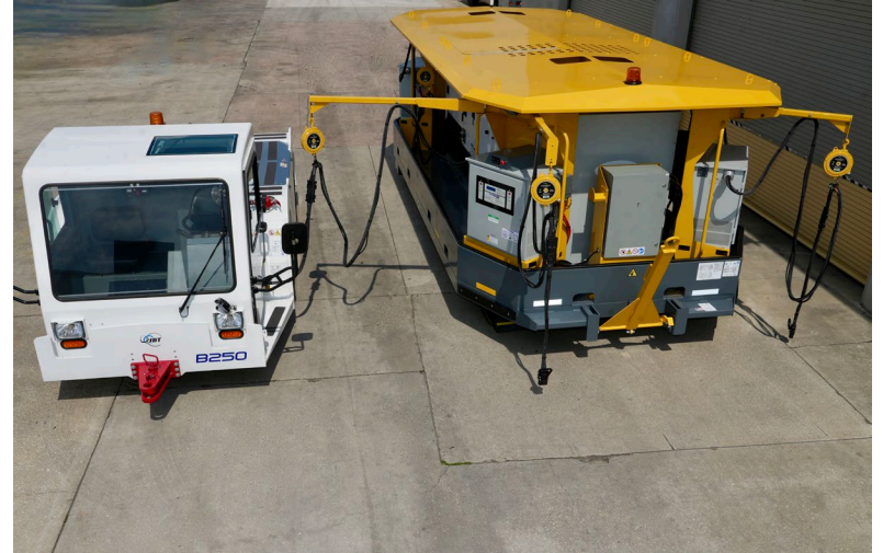
Oshkosh AeroTech Tractor & AmpCart Towable Charging Platform
