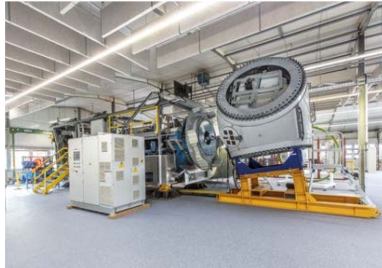
Working model of a hub for training Service technicians at the Technical Training Center, Hamburg, Germany
