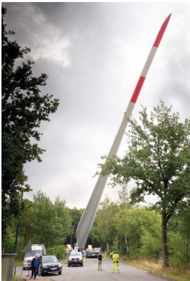
Transporting a 73 m rotor blade for a Delta4000 system is a challenge
