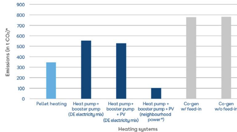
WP = heat pump, PV = photovoltaic system, CHP = combined heat and power plant, CHP = combined heat and power generation.
