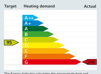
The Energy Indicator calculates the approximate heat and energy use of a building (see "Actual") and simulates the consequences of restoration measures (see "Target")
