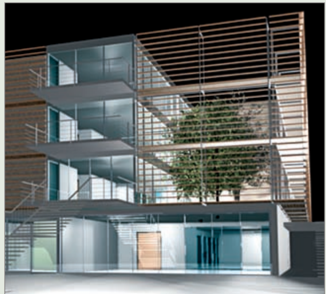
3D model: A virtual building model offers an overall view from all angles and can be used to obtain all kinds of information on the building such as, for example, the required quantities.
