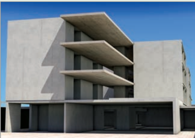
Structure model: Civil engineers are primarily interested in the load-bearing components. In the 3-D model details such as windows and doors can be hidden at the touch of a button.
